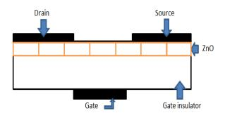
Figure 1. Cross-sectional view of ZnO TFT
